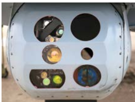
The GOES-451 multi-sensor payload is used for both targeting and night flying/navigation. (Photo: author)
